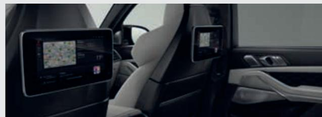
□ Rear-seat Entertainment Professional includes two separate high-resolution 10.2" colour screens with touch function that can be tilted and a Blu-ray drive. In this way, it becomes possible to use navigation and internet functions while driving (if a mobile phone contract exists). Additionally, a USB port and connections for MP3 players, game consoles and headphones (even wireless) are included.
