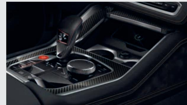
■ The 8-speed M Steptronic transmission with Drivelog offers numerous shifting options: from extremely dynamic to highly comfortable, manual or automatic.
