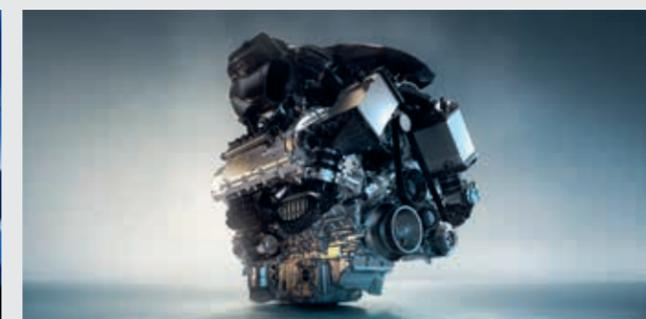
■ The latest version of the high-performance BMW M TwinPower Turbo 8-cylinder petrol engine guarantees performance in keeping with the latest standards. The high-revving unit develops an output of 460 kW (625 hp). The two turbochargers stand out thanks to their cross-cylinder bank exhaust manifold with optimum response characteristics. The V8 engine is also designed for extreme loads on the race track.
