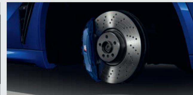
■ Thanks to the use of various materials, M Compound brakes achieve outstanding deceleration values and are extremely stable and highly durable. They also weigh less, which has a positive impact on agility, dynamics and acceleration. The Blue metallic brake callipers with the M designation are the hallmark of these high-performance M specific brakes.
