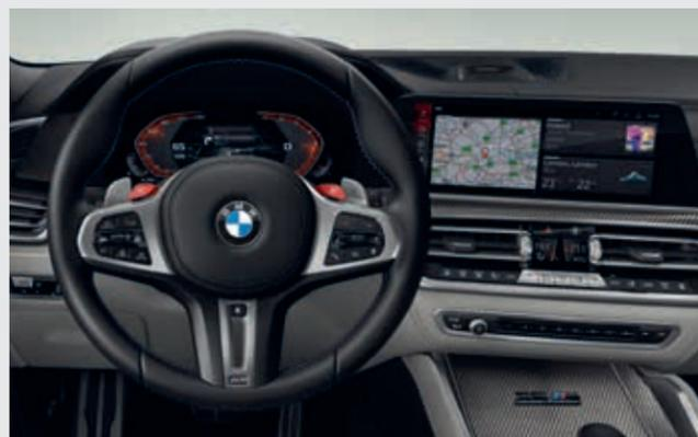
■ The BMW Live Cockpit Professional with navigation function includes two high-quality displays consisting of a high-resolution 12.3" Control Display that can be operated by touch and a fully digital 12.3" instrument display.
