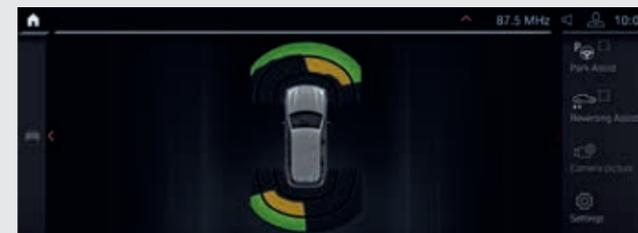
□ Parking Assistant Plus makes parking and manoeuvring the vehicle easier. It features among others the Surround View system including Top View, Panorama View, Remote View 3D, as well as a lateral parking aid, the emergency braking function Active Park Distance Control, Parking Assistant with longitudinal and lateral guidance and Reversing Assistant.
