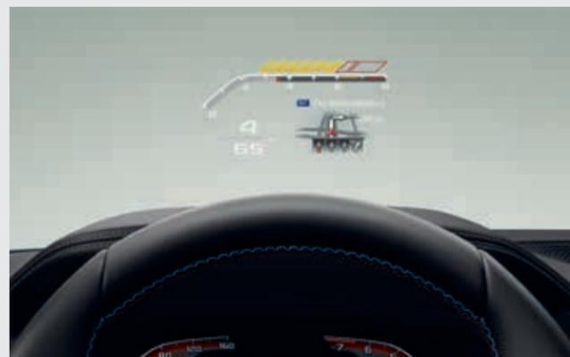
■ The full-colour BMW Head-Up Display<sup>1,\*</sup> incl. M specific display projects all information relevant to the journey directly into your field of vision, allowing you to fully concentrate on driving. Information such as the current speed and, depending on the equipment, navigation directions, Speed Limit Info including no-overtaking indicator, along with telephone and entertainment lists are displayed.
